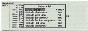
Screenshot 7: setting up the list of views that you can move to when pressing the Diamond key
