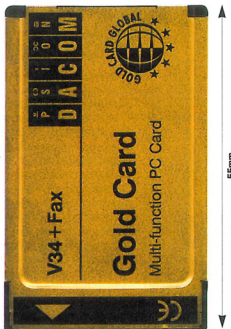
One for all: the Gold Card Global requires only the correct mobile phone kit to give it GSM capability as well as land-line and fax
